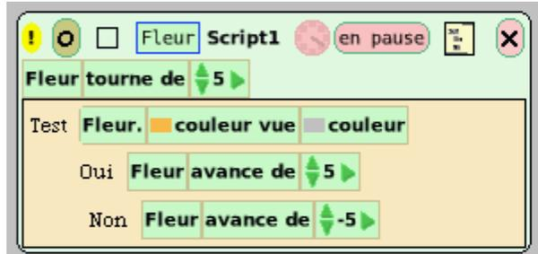
Block languages like Scratch and Etoys represent imperative language grammar and elements into tactile objects. Blocks can be dragged and snapped together, can be clicked to run, and visually display run-time status like errors and execution. This is an aid to comprehension and sharing (Repenning and Ambach 1996). Visual AgentTalk also allows blocks to be dropped onto objects:
